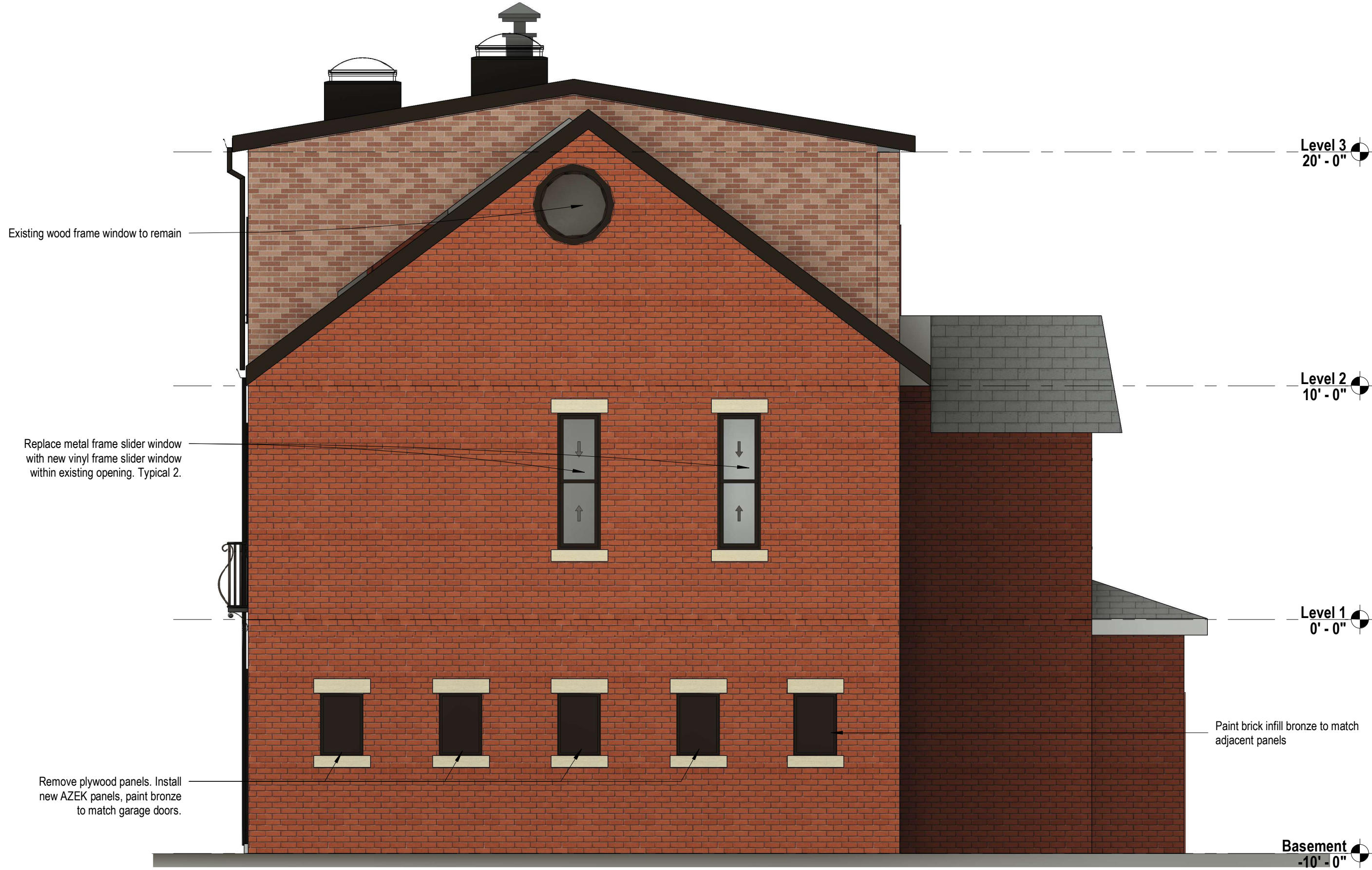
4 West Building Elevation 1/4" = 1'-0"
