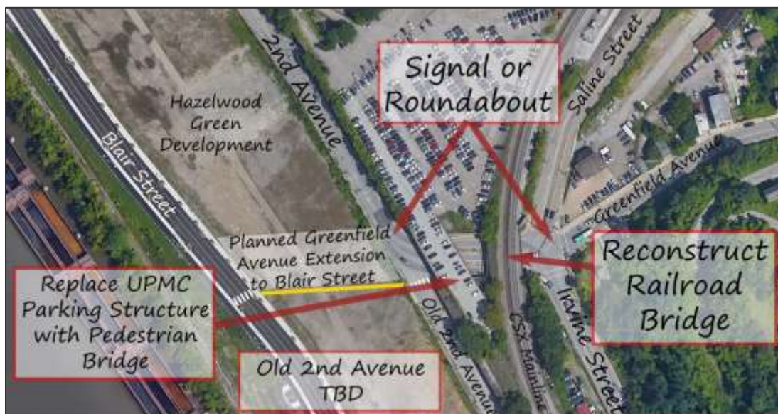
Exhibit 3-20: Reconstruction of Irvine St/Greenfield Ave/Saline St/Second Ave with Pier Removal
