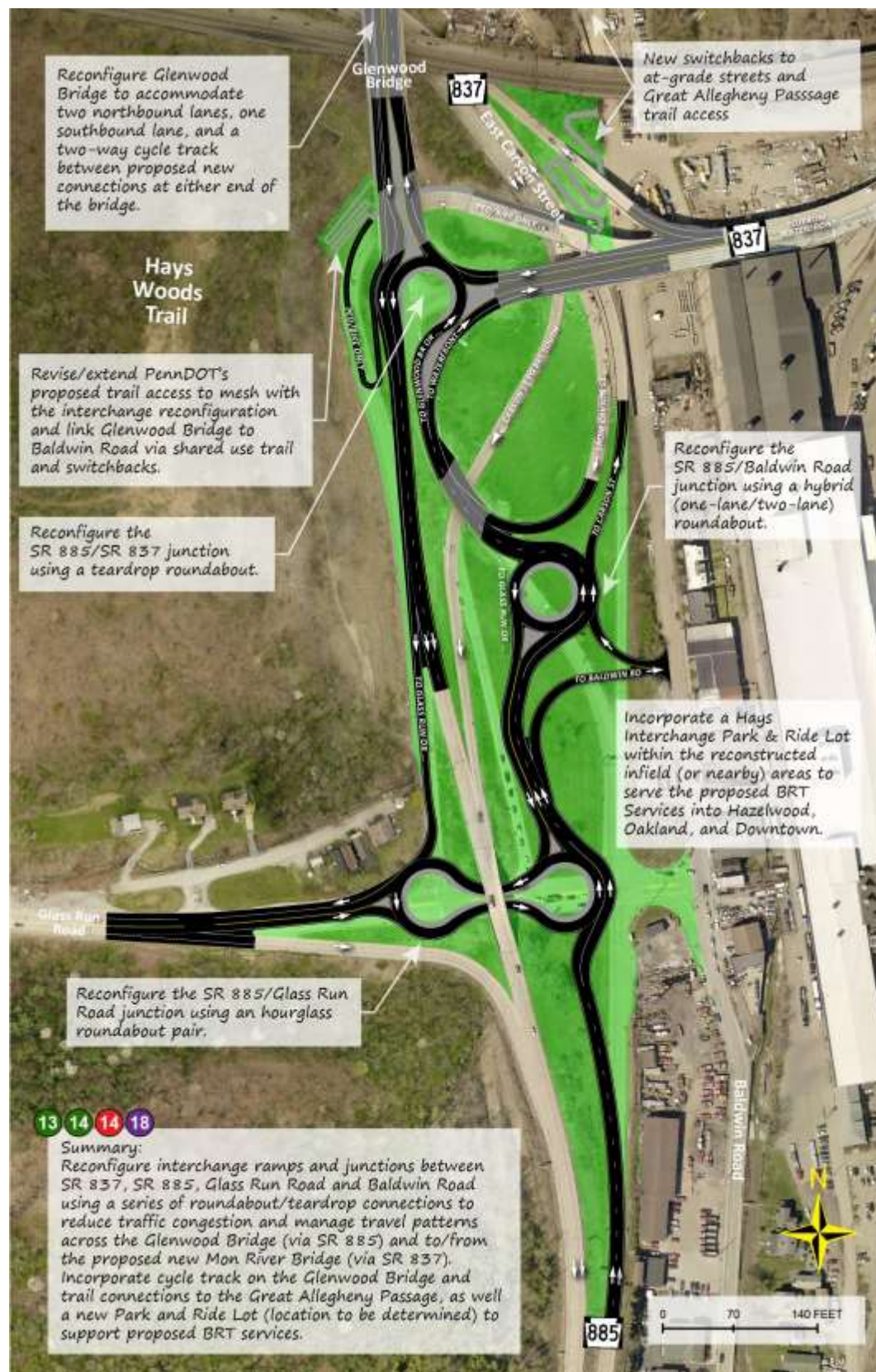
Exhibit 4-13: Multimodal Improvements to Glenwood Bridge and Hays Interchange (Option A)
