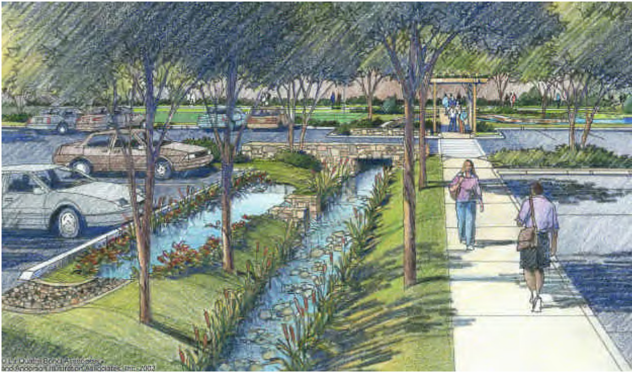
Typical parking lot incorporating ecological techniques including: bio-swales, porous paving and native plant materials resulting in a more natural garden setting.
