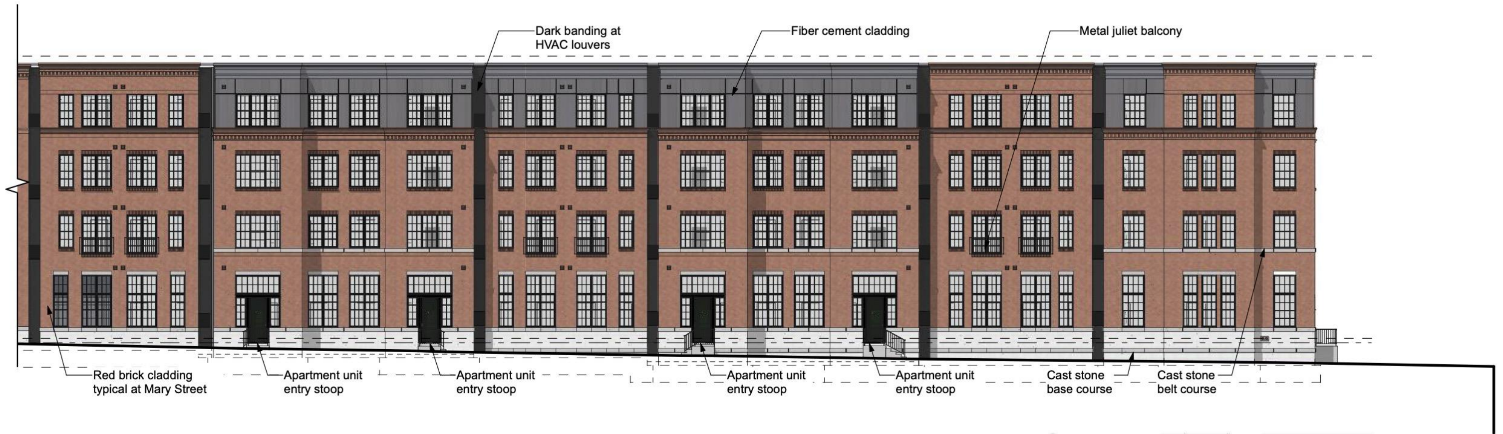
Apartment North Facade (Mary Street) - West Wing
