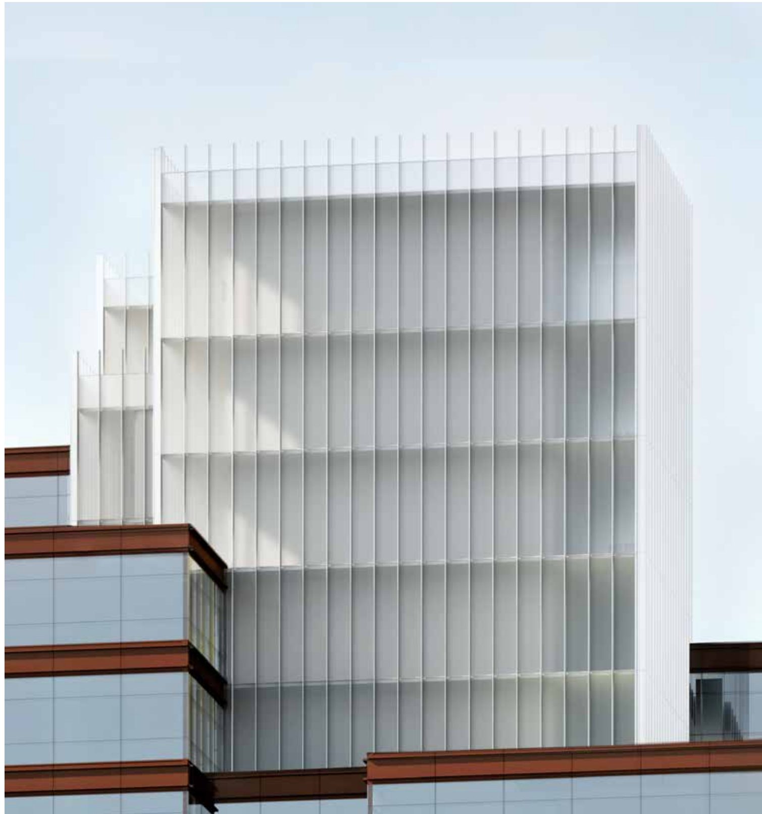
FRITTED GLAZING SYSTEM AT BULKHEAD
