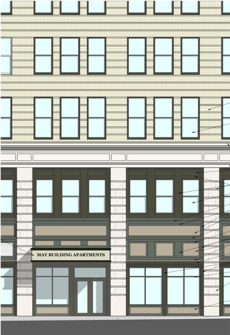
EXISTING BRICK (TO BE REPAIRED WHERE REQUIRED AND CLEANED)
